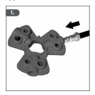
Disconnect the compressed air connection and insert the connector according to its size into one of the appropriate openings of the compressed air connection lockout device.
